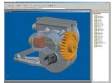
Differential displayed in Autodesk Inventor
